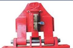
This system is used to fix the cargo wagon during loading and unloading.
